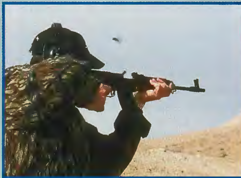
The camera catches an empty 7.62x39mm case being ejected from the VZ2000 a millisecond after Gil Angelotti fires the rifle off-hand. Recoil was light, and the rifle never malfunctioned.
